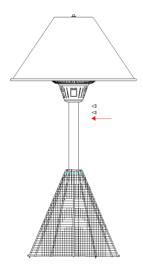
6. Pull the power cord gently out of the base as much as possible. Fix the power cord under the weighted base using the supplied 4pcs M4 nuts.
